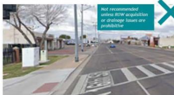
Attached Sidewalk - 8' wide
