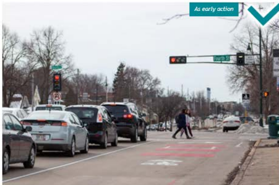
Transit bypass lanes (dedicated lanes for bus approaches to intersections) at key locations, coupled with transit signal priority 'queue jumps'
