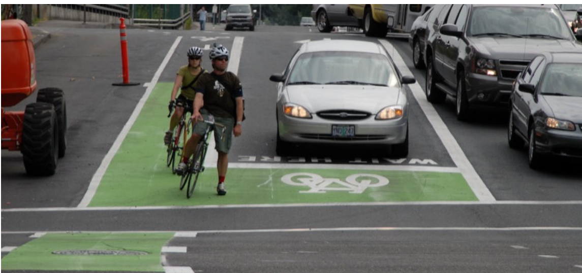
Bicycle Boxes help improve the visibility of people bicycling at intersections. (Photo Credit: Bike Portland)
