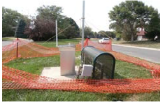
The old weather station and controller. The weather station is mounted to the pole.
