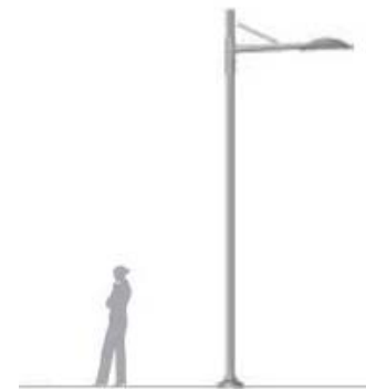
Pedestrian pole with custom extension arm
