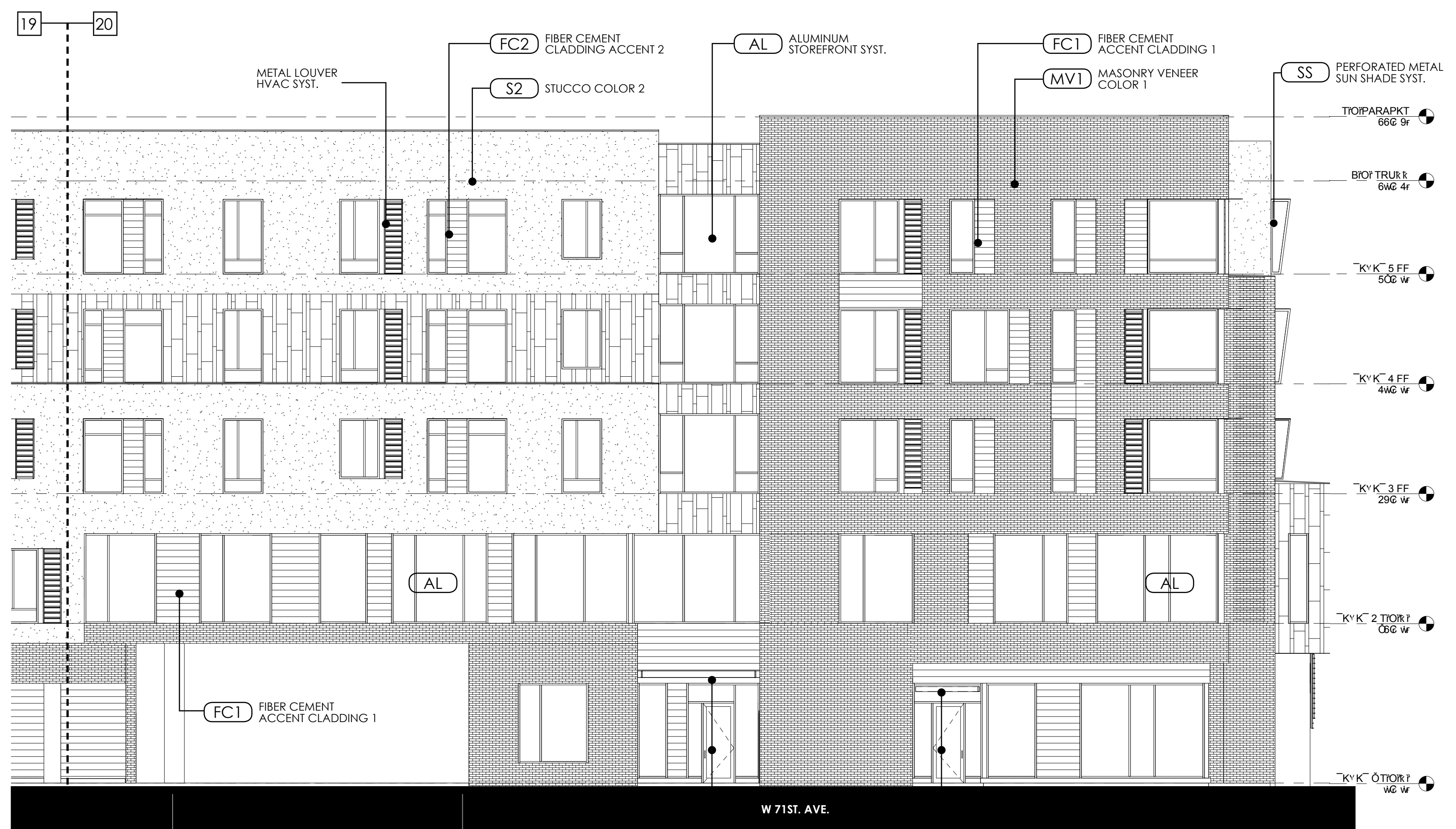
19 20 METAL LOUVER HVAC SYST. FC2 FIBER CEMENT CLADDING ACCENT 2 S2 STUCCO COLOR 2 AL ALUMINUM STOREFRONT SYST. FC1 FIBER CEMENT ACCENT CLADDING 1 MV1 MASONRY VENEER COLOR 1 SS PERFORATED METAL SUN SHADE SYST. TPO/PARAPKT 66G 9f BROF TRUK R 6WG 4f KYK 5 FF 50G Wf KYK 4 FF 4WG Wf KYK 3 FF 29G Wf KYK 2 TPO/P 06G Wf KYK 0 TPO/P Wf Wf W 71ST. AVE. GARAGE ENTRANCE BUILDING ENTRANCE WITH PAINTED METAL CANOPY SYST. & INTEGRATED DOWNLIGHT COMMERCIAL ENTRANCE WITH PAINTED METAL CANOPY SYST. & INTEGRATED DOWNLIGHT PARTIAL SOUTH ELEVATION 1/8" = 1'-0"
