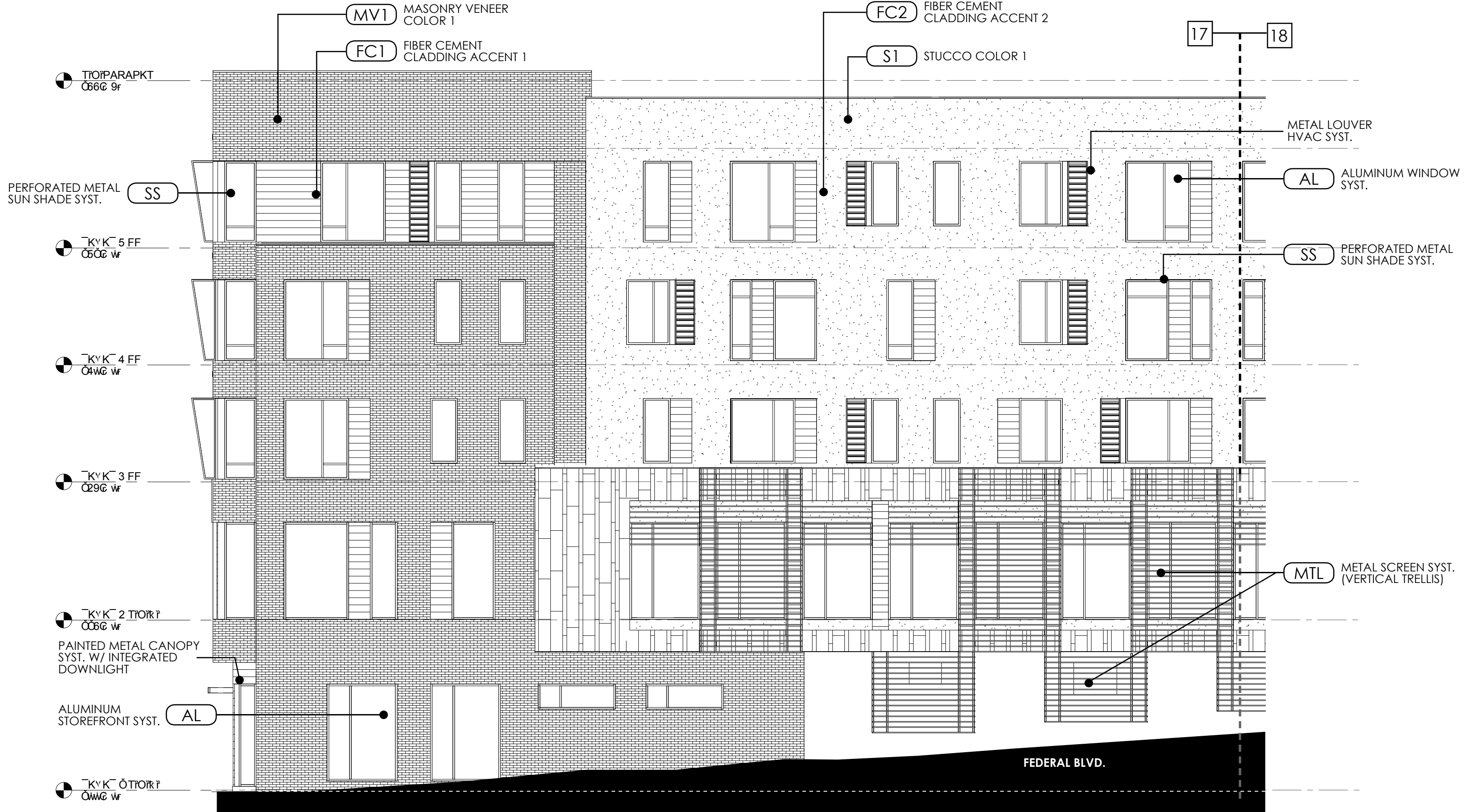
PARTIAL EAST ELEVATION 1/8" = 1'-0"
