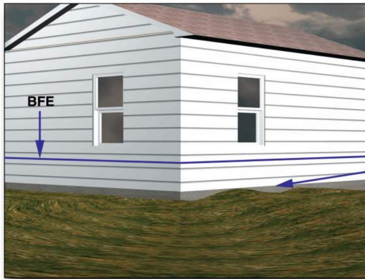
Figure 9 Technique 3 – Lift the entire house, with the floor slab attached, and build a new foundation to elevate the house.
